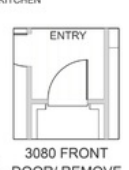
3080 FRONT DOOR/ REMOVE TRANSOM
