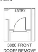
3080 FRONT DOOR/ REMOVE TRANSOM
